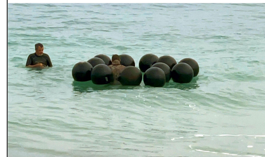
Experimental model of concept with 0.5m diam spheres made with recycled pearl farm floats.
